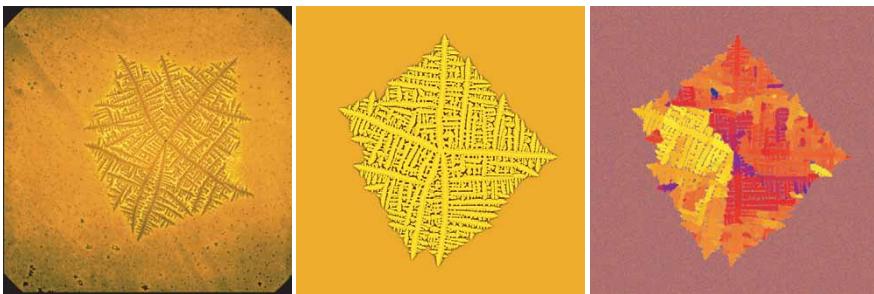
Figure 6. 'Dizzy' dendrite in experiment (left) and phase field simulation (composition: centre; orientation: right).
