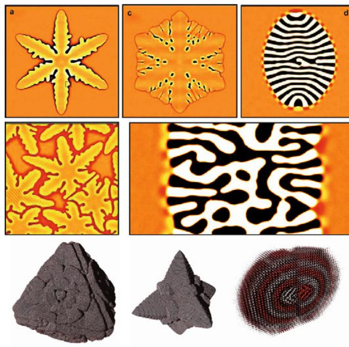
**Fig. 16.** Dendritic and eutectic growth in 2D (first row [75]; second row [76] and [51]) and 3D (third row: bcc and fcc dendrites [51], and bcc eutectics [51]) in the binary 1M PFC model.
